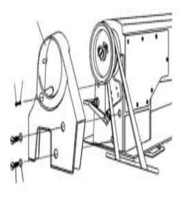
Check whether the belt cover is attached to the table
